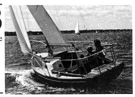
Quickstep 24 is a coastal cruiser designed by Ted Brewer. Renowned for its comfort and performance the Quickstep
