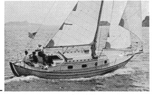
The Gillmer 28 is comfortable and roomy. The modified full-keeled hull has the "feel" of a much larger displacement yacht, yet she is quick and responsive in any condition. The Gillmer 28's cutter rig performs well even in light air often surprising "modern" designs with her spirit.
